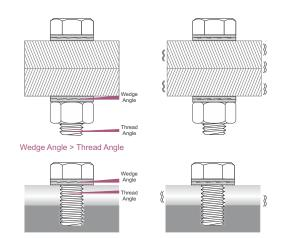
Note: the washers are always used in pairs. For through holes two pairs of Durlok washers should be used. For studbolt Durlok washers lock the nut. Durlok washers must not be used with other flat washers.
